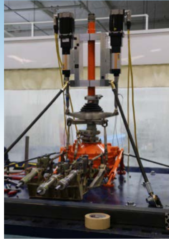
Main Rotor Control System
